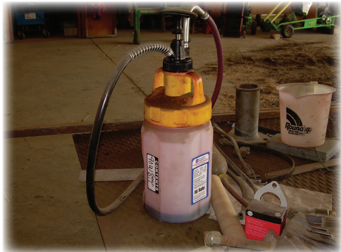
Xpel pump used to dispense LE's Duolec Industrial Gear Oil (1605).
